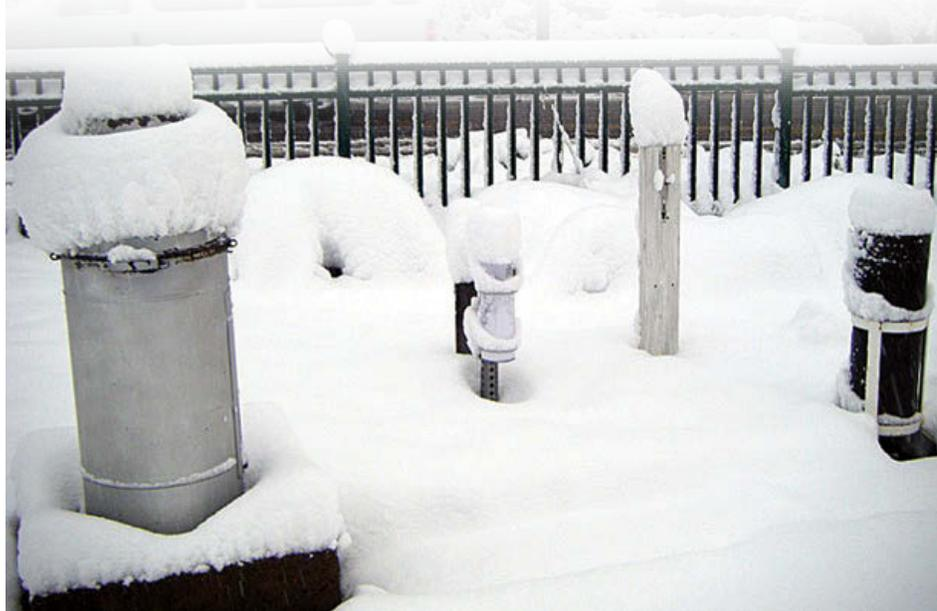
Figure 1. Most precipitation gauges do not measure snow very accurately.
