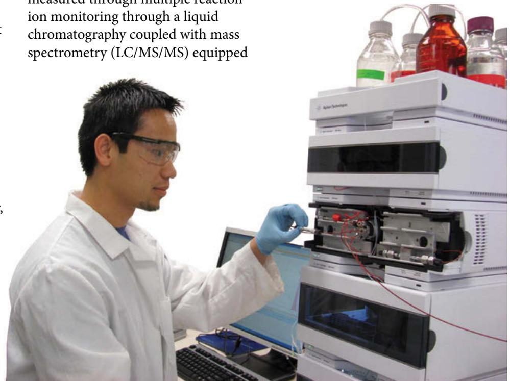
*Victor Sam sets up the HPLC (High Performance Liquid Chromatography) for microcystin-LR analysis. GC & LC/MS/MS analysis was done at the Center for Environmental Medicine Analytical Lab at Colorado State University.*
